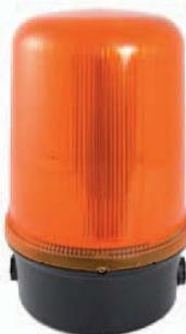
Strobe lights use a xenon discharge tube and an electronic circuit which discharges a capacitor through the xenon tube to produce a short, high intensity burst of light. Although the strobe light is emitted through 360°, it is often most intense in one direction.
