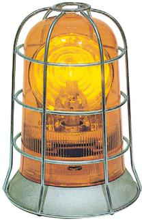
The Rotating Beacon uses a rotating reflector, driven by a small electric motor, which revolves around a centrally located lamp. The effect is a beam of light which rotates through 360° usually at a speed of 180rpm for industrial beacons. The rotating beacon is available with either conventional filament lamps or halogen lamps.
