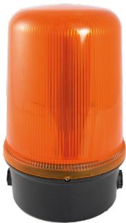
Strobe lights use a xenon discharge tube and an electronic circuit which discharges a capacitor through the xenon tube to produce a short, high intensity burst of light. Although the strobe light is emitted through 360°, it is often most intense in one direction.
